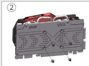
Unscrew the GPU backplane screws
