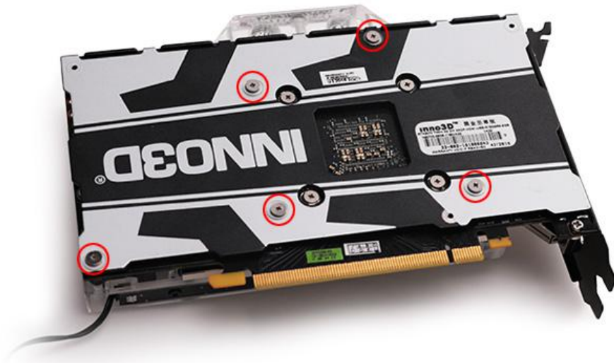
7.Mounting the shown in the picture Red Position Screws
