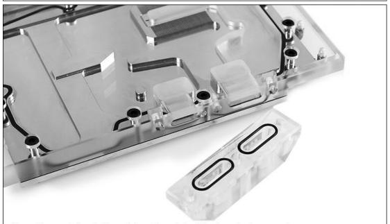
Press the seal ring in the rubber ring slot of the terminal connector (Little tips: It will be easier to install if you gently pull the seal ring before installation)
