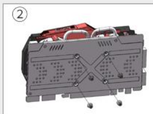
拆除原装显卡背板螺丝
